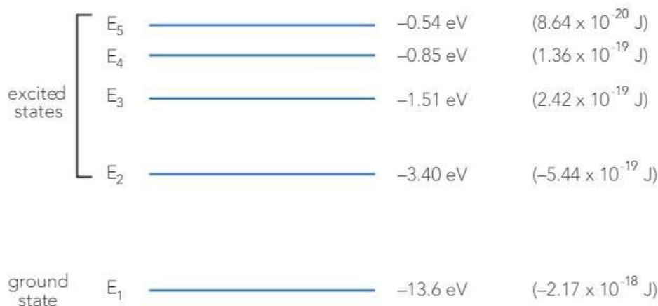
Figure 3.8 Energy levels of a hydrogen atom. It can be shown that E_n \propto \frac{1}{n^2} , n being the level number.
