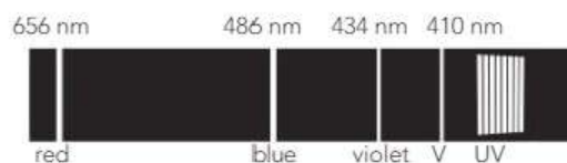
Figure 3.10 Hydrogen line emission spectrum. Only 4 lines are in the visible region.
